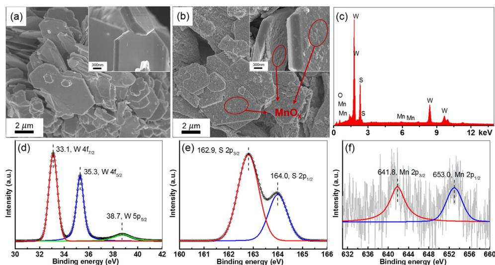
**Fig. 1.** (a, b) SEM images of WS<sub>2</sub> (a) and MnO<sub>x</sub>/WS<sub>2</sub> (b), inset of (a) and (b) are the magnified SEM images of WS<sub>2</sub> and MnO<sub>x</sub>/WS<sub>2</sub> respectively. (c) EDS spectrum of MnO<sub>x</sub>/WS<sub>2</sub>. (d–f) XPS scan of W 5p and W 4f (d), S 2p (e), and Mn 2p (f) for MnO<sub>x</sub>/WS<sub>2</sub>.
