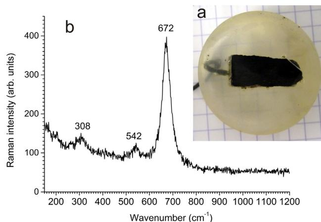
**Fig. 2.** (a) Photograph of the magnetite electrode and (b) typical Raman spectrum obtained during analysis of its surface.
