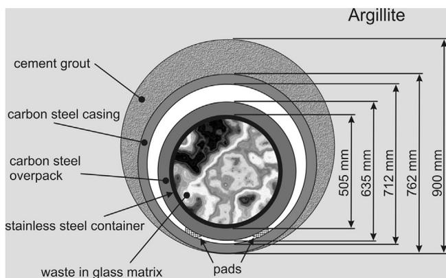
**Fig. 1.** The envisioned multi-barrier concept for the French disposal of high level nuclear waste: cross-sectional view.
