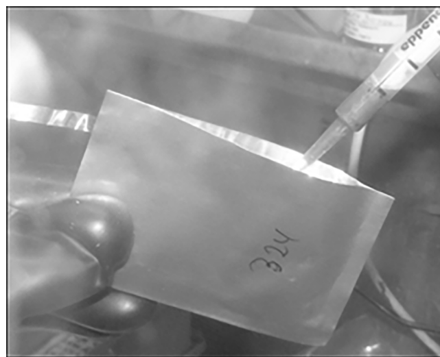
Fig. 2. Pouch bag cells are opened after a specified number of cycles (25, 40, 50 and 65, respectively) and 1,4-dioxane is inserted. The solution is then extracted from the cell by a syringe.
