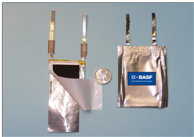
Fig. 1. Standard pouch bag test cells.
