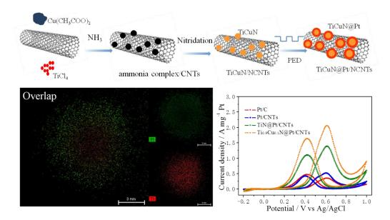
The novel core-shell Ti<sub>0.9</sub>Cu<sub>0.1</sub>N@Pt/CNTs catalyst exhibits high methanol oxidation reaction activity and durability.
