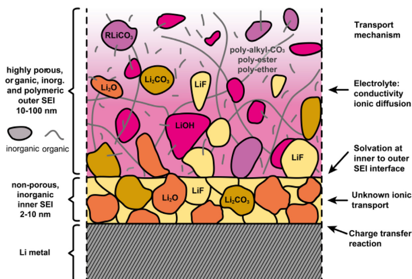
Fig. 1. Schematic of SEI and involved processes: sketch of the solid-electrolyte interphase that forms on alkali-metals with an inner inorganic non-porous layer and an outer highly-porous layer of organic, inorganic and polymeric electrolyte reduction products, transport processes are indicated on the right side including surface reactions, ionic transport through the inner SEI, solvation at the inner-outer SEI interface and electrolyte transport through the outer porous SEI.
