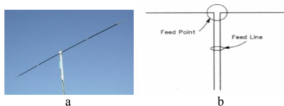
Figure 1. Dipole Antenna. a dipole antenna in reality [9] b dipole antenna model [5]
