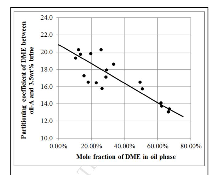
DME-partitioning between a live oil and 3.5wt% brine at 343 K: marker points correspond to in-house experimental data measured at 10,000-14,000 kPa; solid lines correspond to the computed results using PR78 EOS with Huron-Vidal mixing rule at 12,000kPa.
