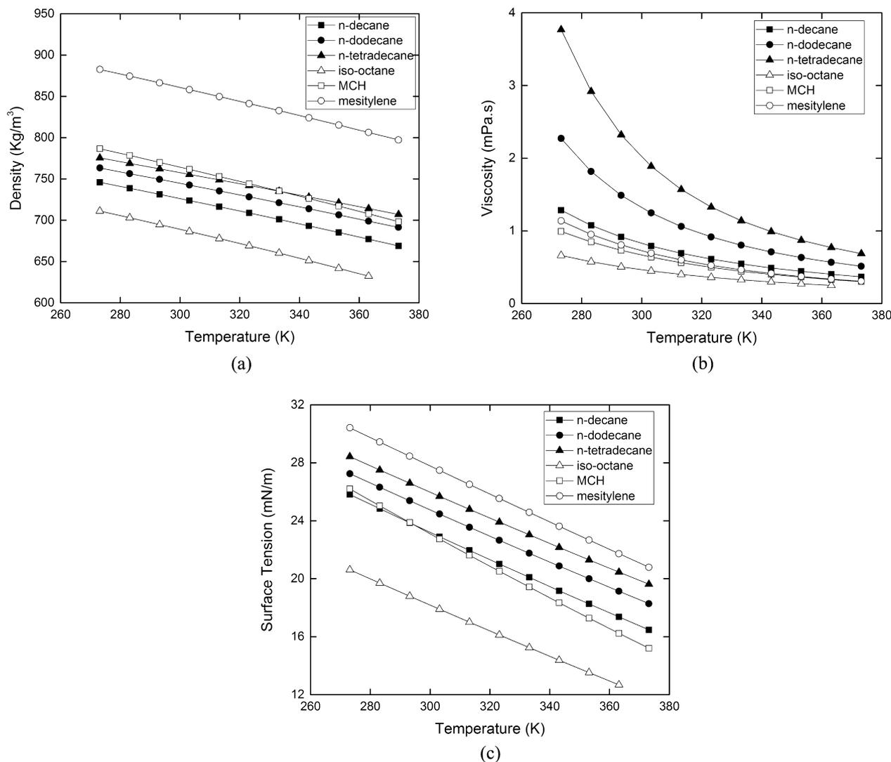
**Fig. 1.** Physical properties of the neat surrogate candidates as a function of temperature; (a) density, (b) dynamic viscosity, and (c) surface tension.
