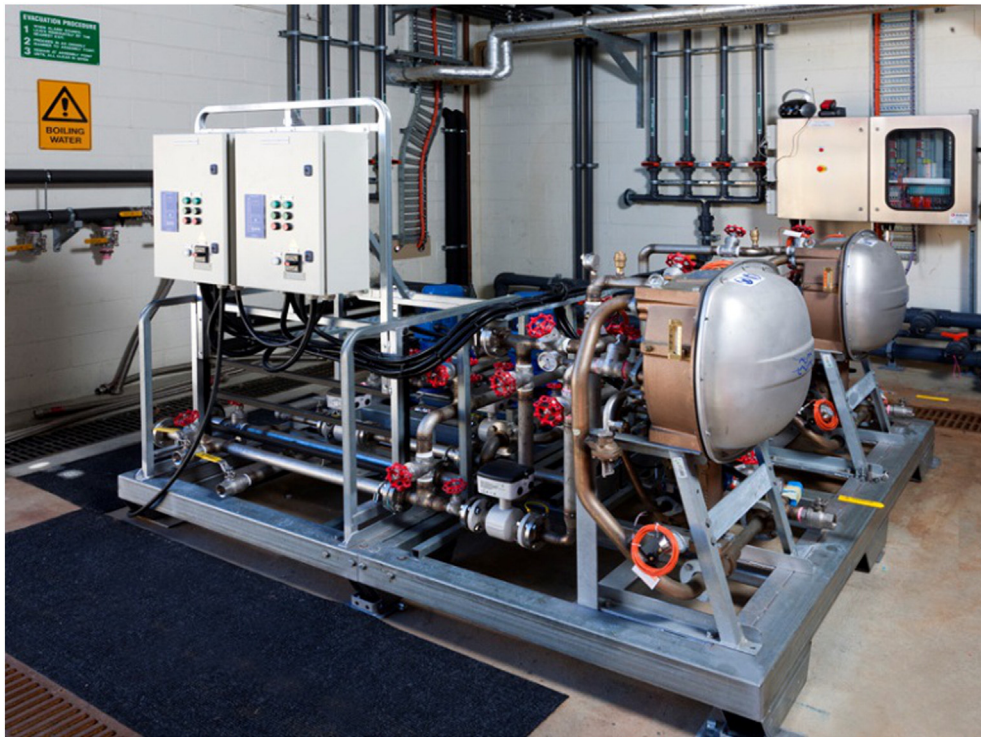
Fig. 1. The two serially connected Alfa Laval's single-effect rising film plate evaporators modules (JWP-16-C Series) (Christ et al., 2015).
