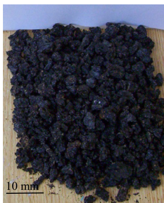
c. Photo of volcanic scoria aggregates as received
