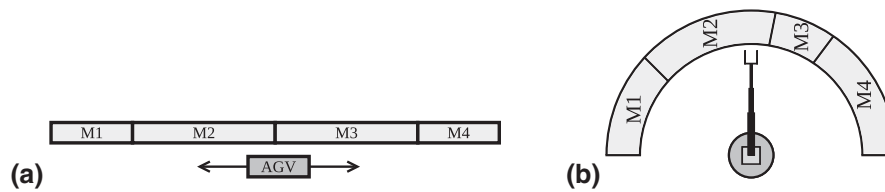
Fig. 1. In (a) an AGV transports parts between the machines moving in both directions along a straight line. In (b) a material-handling industrial robot carries parts between the machines.
