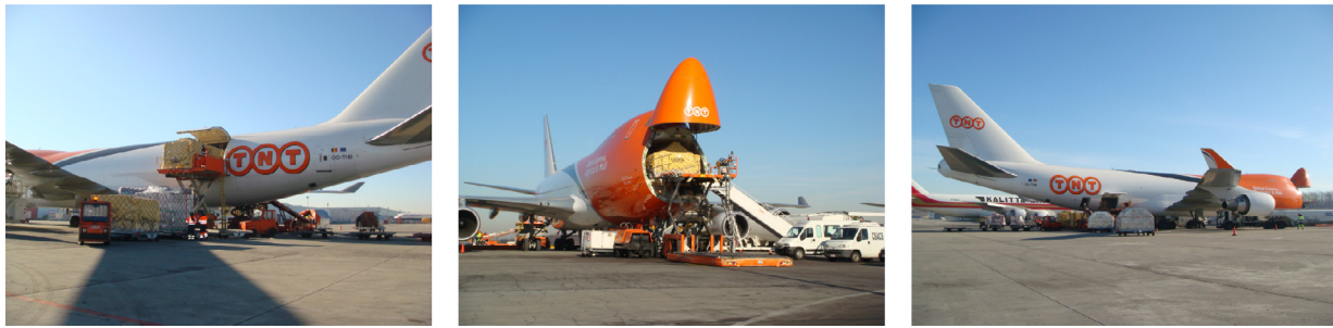
Fig. 1. ULD loaded through main deck side cargo door (left), through nose door (middle), and through lower deck side cargo door (right).
