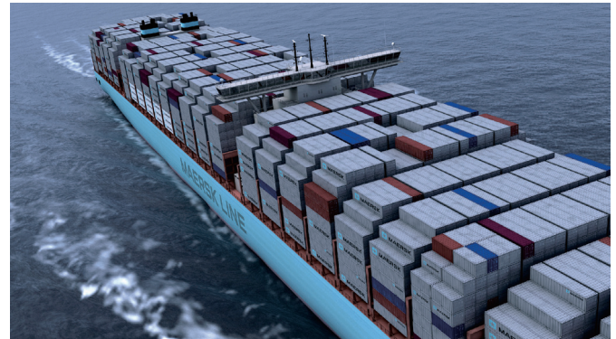
Figure 3. The Triple E. An example of the new generation of large container ships; it is 400 m long and 59 m wide, has a speed of 19 kn and carries 165 000 DWT. ( http://www.maersk.com/en/search?q=Triple%20e&t=images , 12 February 2015)
