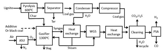
Fig. 1. Schematic of the proposed brown coal pyrolysis-gasification process.
