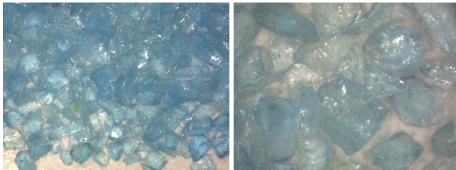
Fig. 1. Crystals of chalcantite from the Kosmurun deposit: left - magnification \times 50 , right - magnification \times 200 .
