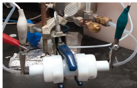
Fig. 1. Graphical and pictorial illustrations of the miniature PEM fuel cell test fixture developed for this work. Left, diagram of the assembled parts that make up the test fixture. Right, photograph of the text fixture in use. For clarity, the bottom photograph is shown without the heating tape that normally surrounds the cell when in use to allow for cell temperature control.
