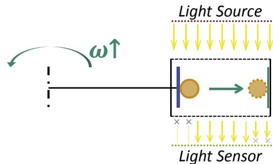
Fig. 2. Scheme of the centrifuge setup: The dough piece casts a shadow, which is recorded.
