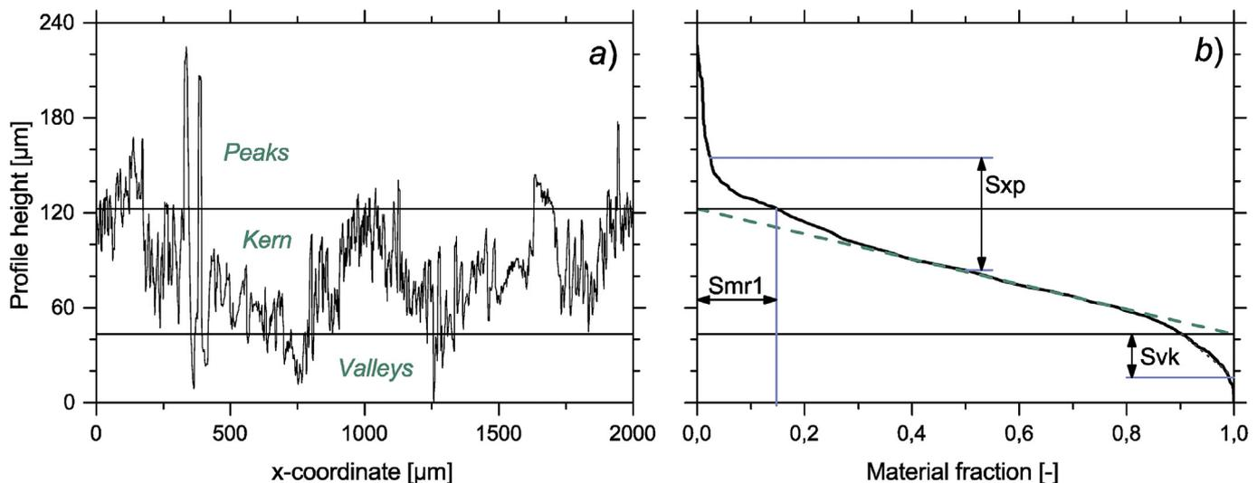
Fig. 1. Surface evaluation according to ISO 25178: From the surface profile (a) the material ratio curve (b) is calculated. The flattest secant spanning 40% defines the kern region; material above constitutes the peaks with their projected surface share  $Smr1$ . Peak Extreme Height  $Sxp$  is read off as the height difference between 2.5 and 50% material fraction;  $Svk$  indicates the Reduced Valley Depth.
