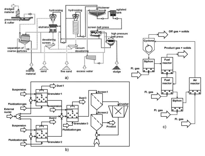
Fig. 1. Examples of solids production processes: soil dewatering and separation [4] (a); granulation (b); chemical looping combustion (c).
