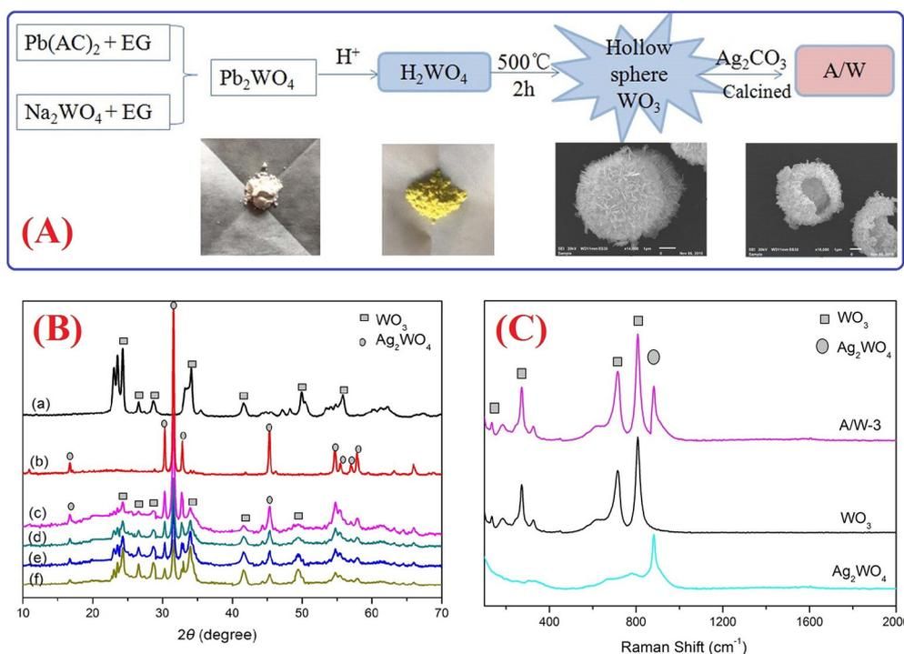
Fig. 1. (A) The synthetic route of hierarchical flower-like hollow structure  $\text{Ag}_2\text{WO}_4/\text{WO}_3$  photocatalyst; (B) XRD patterns of the pure  $\text{WO}_3$  (a), pure  $\text{Ag}_2\text{WO}_4$  (b), A/W-4 (c), A/W-3 (d), A/W-2 (e) and A/W-1 (f); (C) Raman spectra of bare  $\text{Ag}_2\text{WO}_4$ ,  $\text{WO}_3$  and heterojunction structure A/W-3 photocatalyst.
