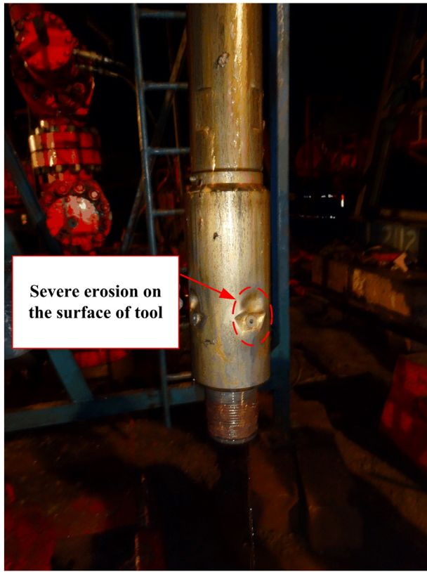
Fig. 1. Image showing severely eroded fracturing tool.
