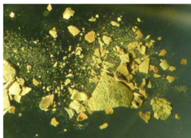
Fig. 2. Precipitate found in T4 degassing column.
