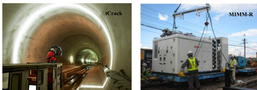
Fig. 1. Typical inspection equipment in subway tunnels.
