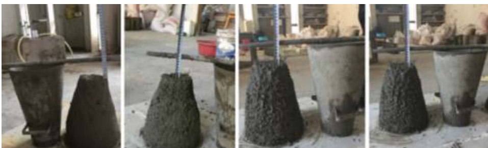
Fig. 1. Slump test for the plain and fibrous mixtures.
