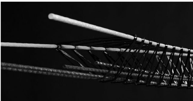
Fig. 1. Filament Wound FRP (W-FRP) reinforcement.
