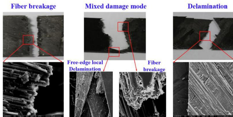
(b) Three typical failure modes
