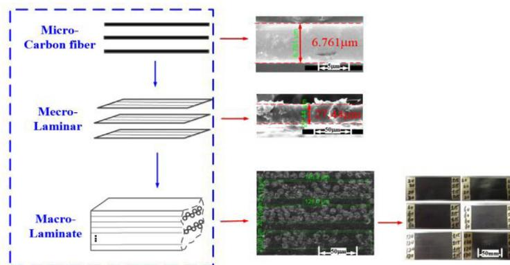
(a) Laminate fabrication and geometry parameter measurement
