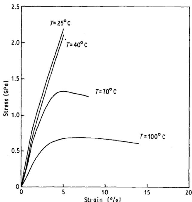
Fig. 1. Stress-strain curves obtained at various temperatures [14].
