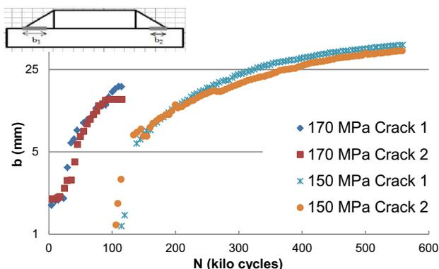
Fig. 1. Disbond length (b) measurements for the type I asymmetric specimens, adapted from [9].
