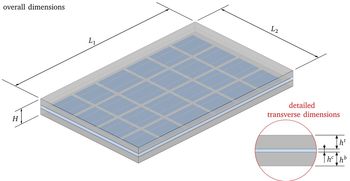
**Fig. 1.** Longitudinal and transverse geometrical measures of the body  $\mathfrak{B}$  mapped by a typical photovoltaic module structure (not to scale).
