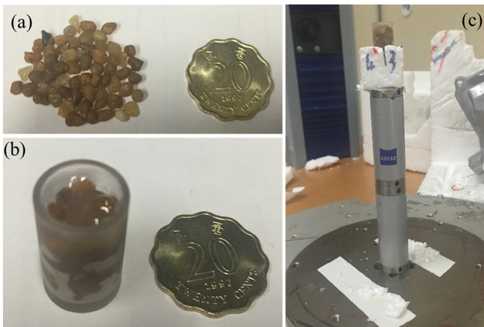
Fig. 1. Preparations for the \mu CT scanning of sand particles: (a) selected LBS particles; (b) microtube specimen containing the LBS particles fixed with silicon grease; and (c) rotation unit base for the microtube specimen subjected to X-ray scanning.
