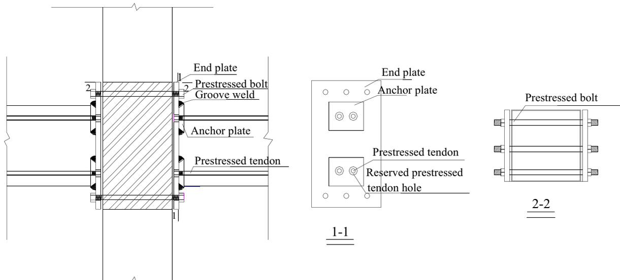
Fig. 1. The detail figures of connection.
