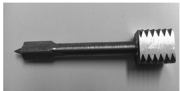
Fig. 1. Novel nail proposed for the Torque Penetrometric Test of historical mortars [25].
