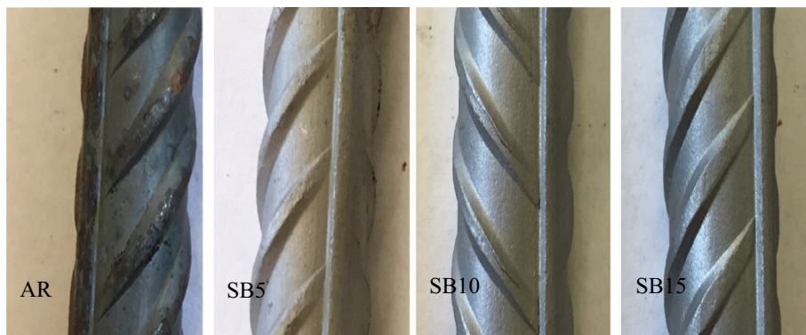
Fig. 2. The surface of steel specimens, before exposure to the pore solution.
