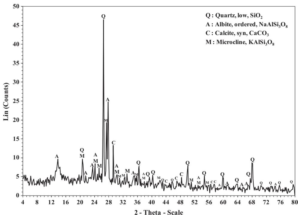
Fig. 2. XRD pattern of meta-kaolin.
