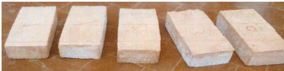
Fig. 1. Geopolymer bricks.
