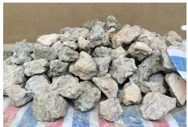
(b) Waste concrete blocks
