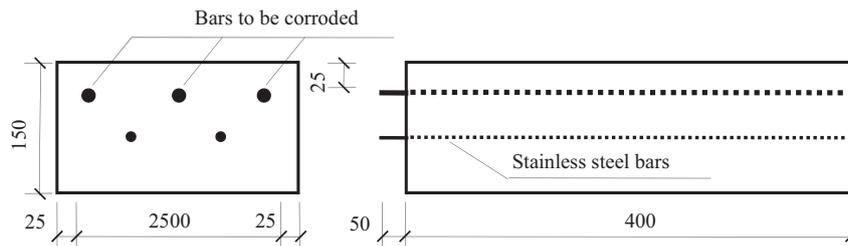
Fig. 1. Geometry of concrete slabs (unit: mm).
