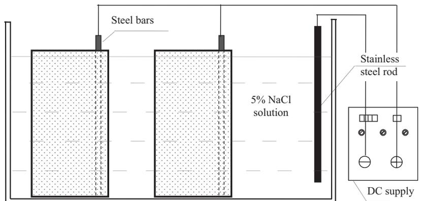
Fig. 2. Full-immersion accelerated corrosion method.
