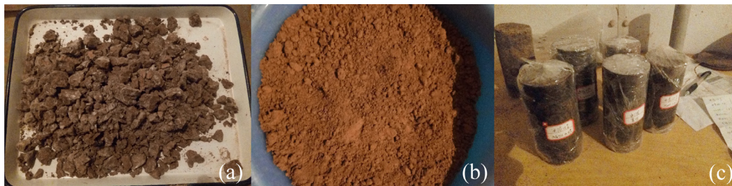
Fig. 1. Sample-preparation procedure in the refrigeration house, (a) frozen soil, (b) crushed frozen soil, (c) samples.
