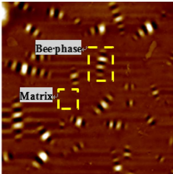
Fig. 1. Microstructures of asphalt binders showing bee phase and matrix phase.
