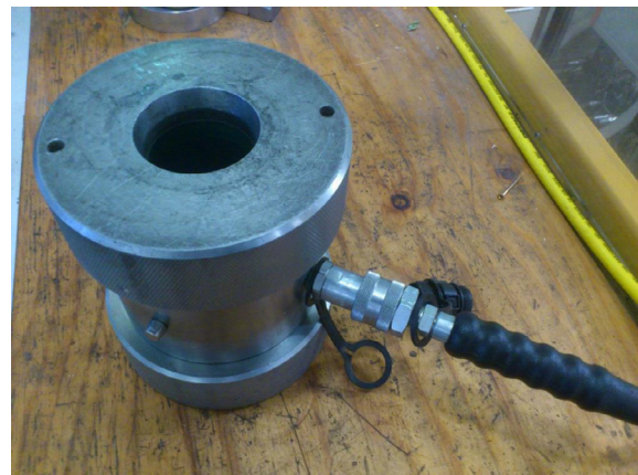
Fig. 2. Hoek cell used for applying active confinement.
