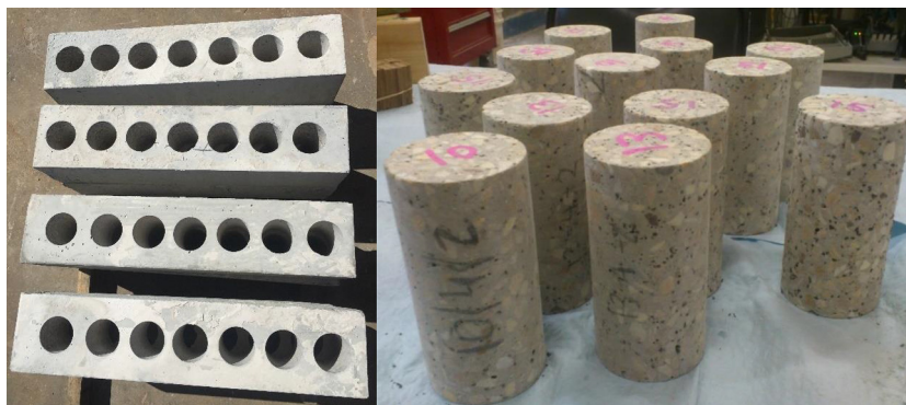
Fig. 1. Cored specimens from the concrete blocks.
