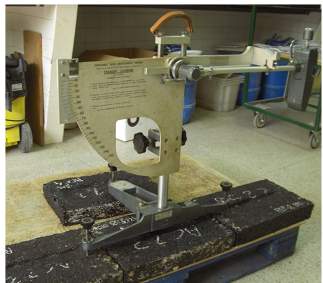
Fig. 2. Evaluation of skid resistance.
