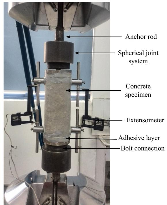
**Fig. 1.** Experimental set-up for cyclic tension test of concrete.
