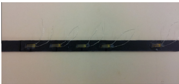
Fig. 1. Strain gauges protected by M-wax coating.
