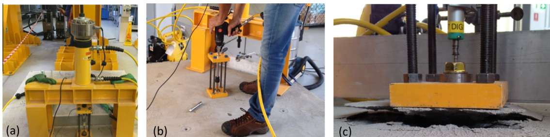
Fig. 2. (a) Reacting frame, load cell, cylinder jack, displacement transducer and fixture, (b) anchor installation and (c) displacement transducer.
