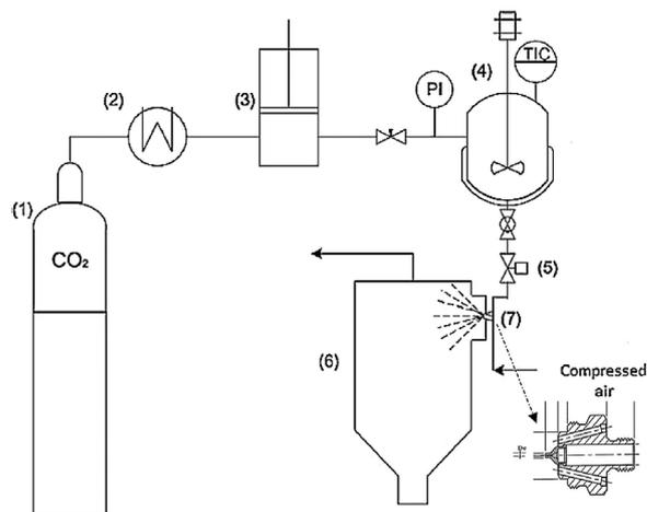
Fig. 1. Experimental setup FAME Separex: (1) carbon dioxide cylinder, (2) cryostat, (3) pneumatic pump, (4) stirred vessel, (5) depressurization valve, (6) cyclone and (7) nozzle  $d = 250 \mu\text{m}$ , with external mixture with compressed air.
