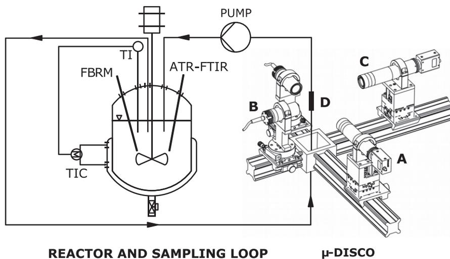
**Fig. 1.** Schematic of the new dual imaging system for crystallization observation ( $\mu$ -DISCO). The suspension flowing from the reactor through the flow channel (D) is back-light illuminated using two telecentric illuminators (B). The suspension is photographed using two digital cameras (A) with telecentric optics (C). The camera, lens and the illuminator system are mounted orthogonally on an optical rail construction.
