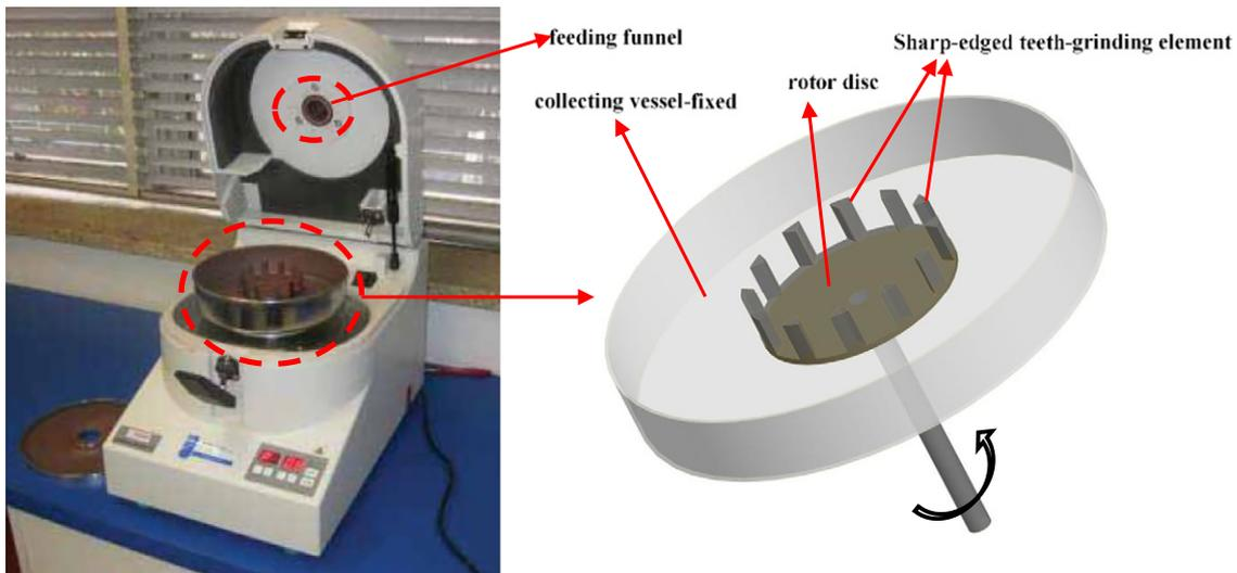
Fig. 1. Details of the impact mill used in the experiments.
