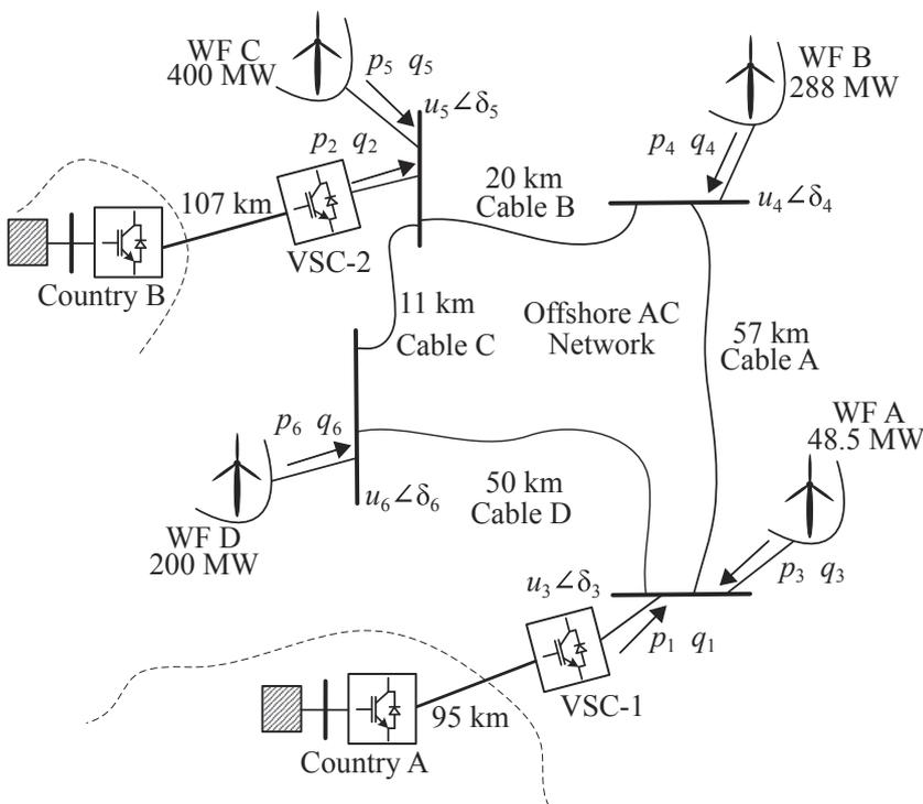
Fig. 1. Configuration of offshore AC network interconnecting two onshore grid using VSC-HVDC system.
