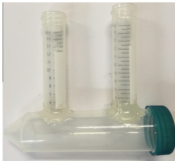
Fig. 1. Layout of the tubular MFC, realized by means of one 50 mL and two 20 mL Falcon test tubes.
