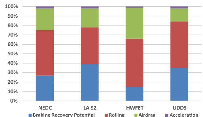
Fig. 1. Energy consumption distribution in driving cycles, with the energy lost in braking shown in blue. (For interpretation of the references to color in this figure legend, the reader is referred to the web version of this article.)
