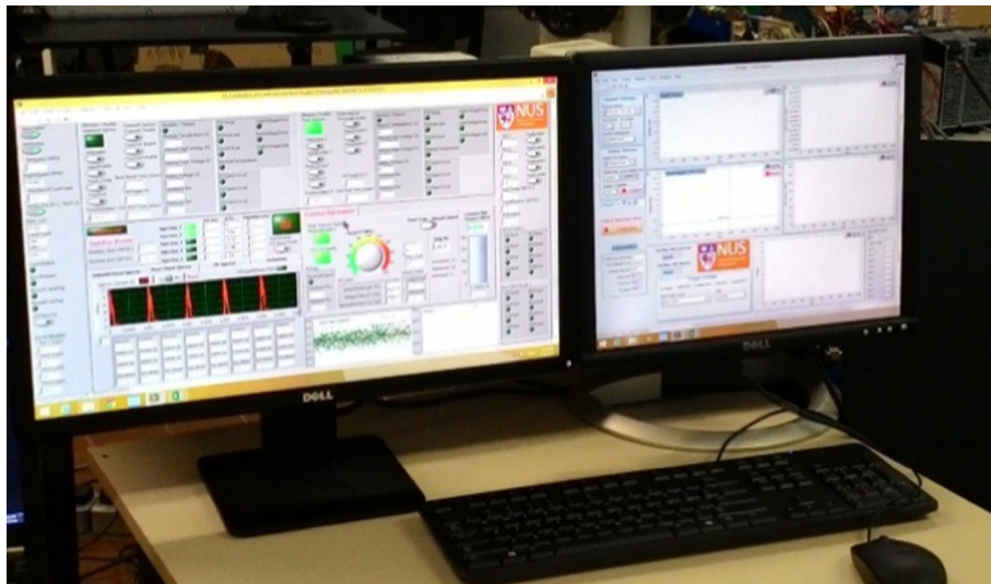
Fig. 2. Built-in-house electronic control system for spray study.
