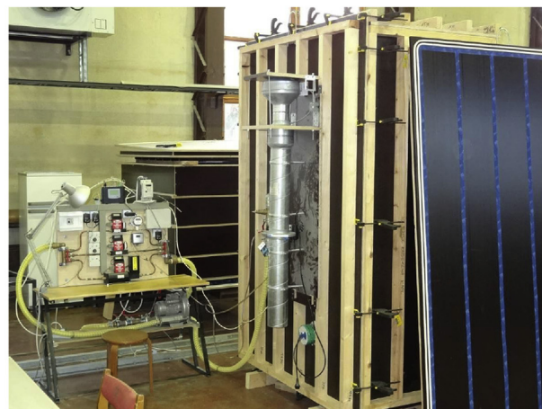
Fig. 1. Test arrangements for the tests of structures in the air leakage test equipment (dimensions in mm).
